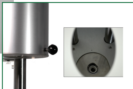
Fig 3. Close-up showing die release knob and inset, looking in mirror at the die.
