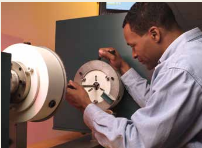
Fig 6. Samples are easily mounted in the patented bi-directional grips.
