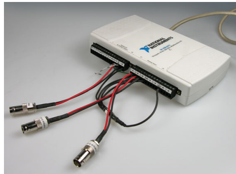
Figure 3. Standard Input/Output box allows data to be taken from multiple sources and channels and supports data transfer to and/or from the Video Extensometer application software.
