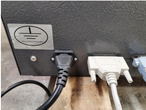
Wire connection with ground wire
