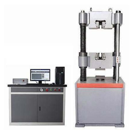
I Equipment name: Computer Control Electro-hydraulic Servo Universal Testing Machine
