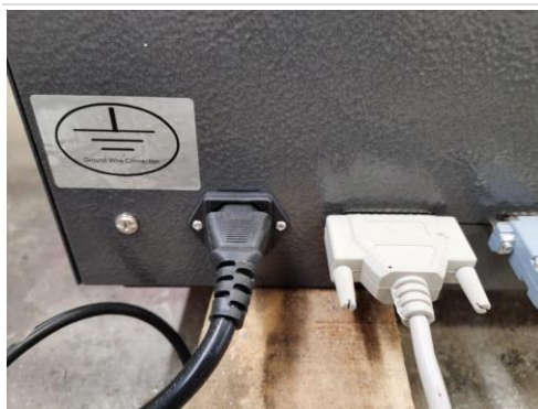
Wire connection with ground wire
