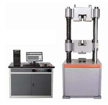
I Equipment name: Computer Screen Hydraulic Universal Testing Machine
